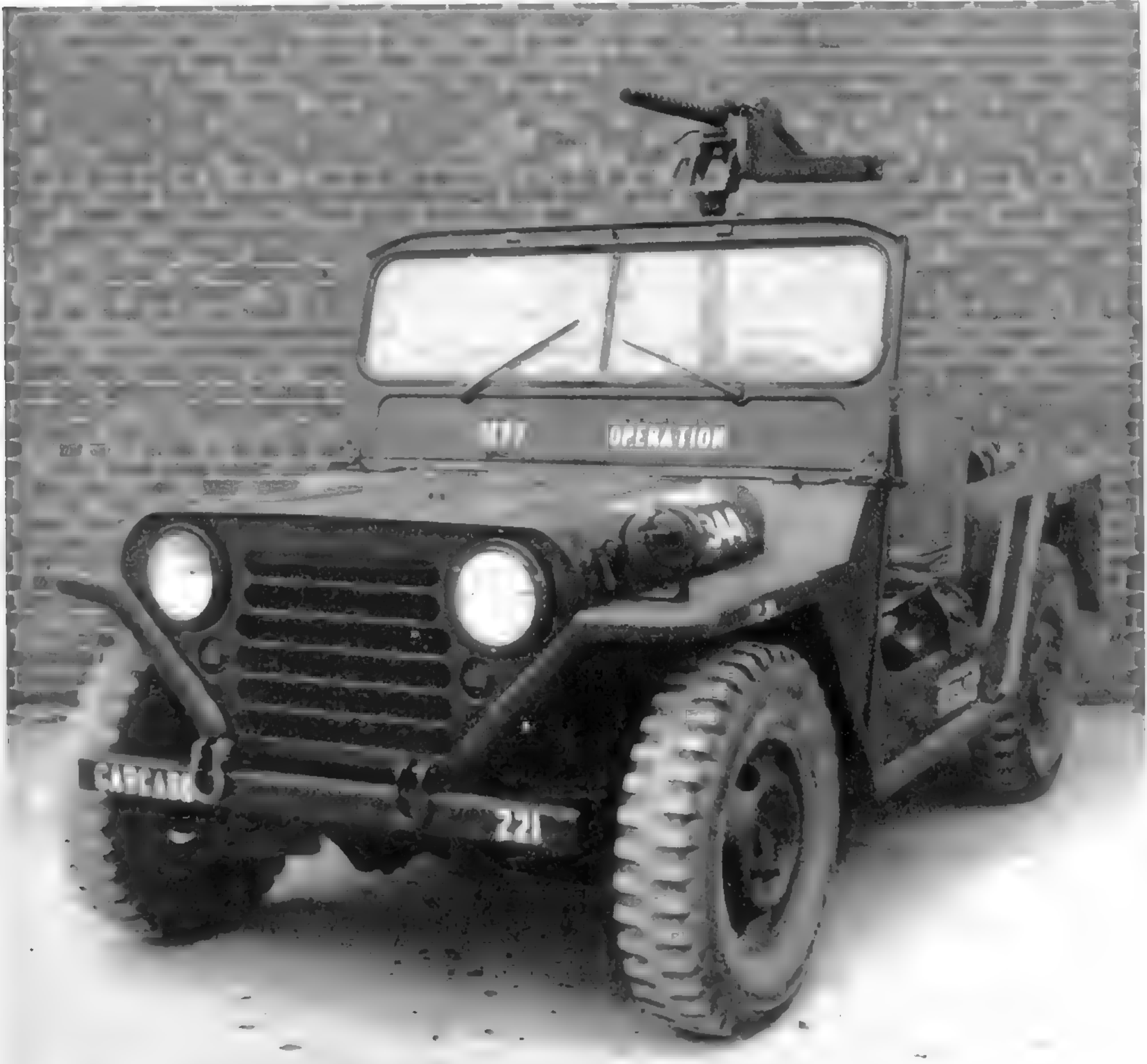
This M151 has been armed with a pedestal-mounted .30-caliber machine gun. The flat fenders and two-piece windshield are characteristics of early models. (Photo courtesy of the Patton Museum)
